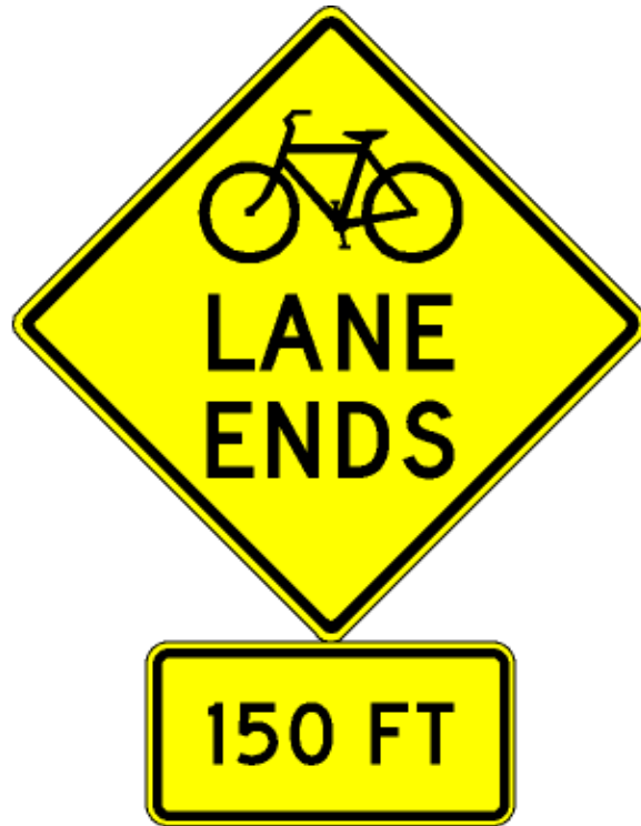
W9-XX Bike Lane Ends Sign + W16-2a Plaque (30" panel, 10" tall bicycle symbol, 5" D text)
